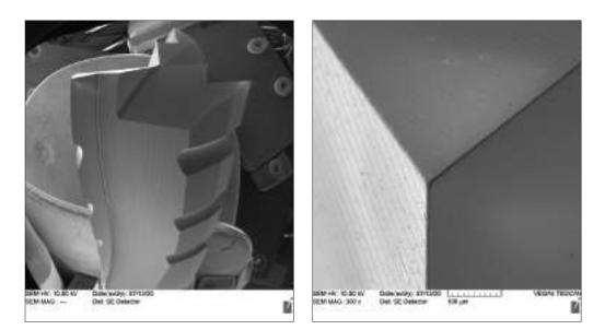
figure 3 - DLC<sup>3</sup> coated endmill under scanning electron microscope
