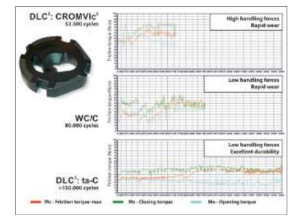
figure 4 Comparison of the frictional torque of different DLC-coatings on a ceramic closure wear element in a water tap [6]
