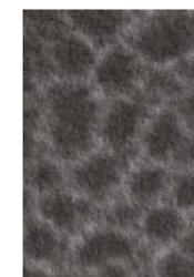
**Nanocomposites (NC)** consist of an adhesion and a core layer. The core layer consists of 2 phases: hard, nanocrystalline grains (e.g. TiN, TiAlN or AlCrN grains) are embedded in an amorphous SiN matrix, which prevents the grain from growing and creates the nanocomposite structure. Column growth is prevented and a fine crystalline/amorphous structure is formed. One example is nACo.
