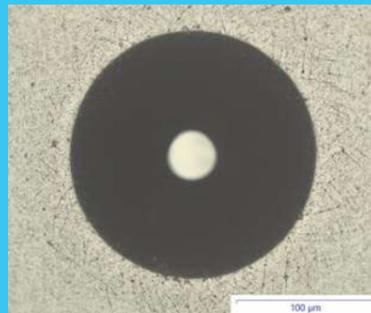
AlCrN, deposited on nitrided substrate
