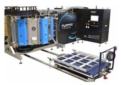
A rail system ensures that the carousel trolley is always correctly aligned with the chamber, thereby making the loading and unloading of loads of up to 1800 kg easy. The height of the custom-designed carousel trolley can be adjusted at the touch of a button.
