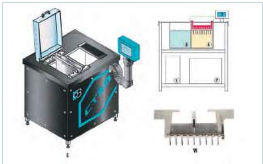
**3 Super-fast decoating with PLATIT's CT-Technology** E: New design of the decoating unit CT20 A: Stripping bath B: Bath for corrosion protection S: Control unit (computer) P: Pulsed power supply W: Tool holder with shank tools (© Platit)
