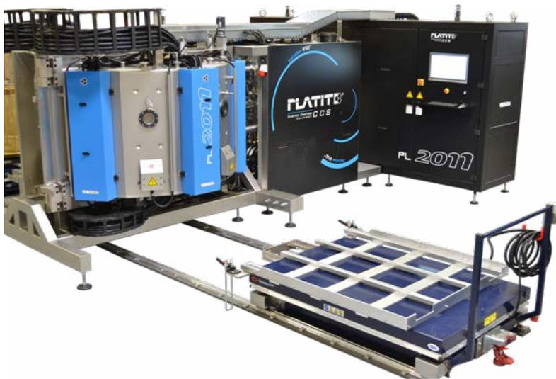
A rail system ensures that the carousel trolley is always correctly aligned with the chamber, thereby making the loading and unloading of loads of up to 1800 kg easy. The height of the custom-designed carousel trolley can be adjusted at the touch of a button.
