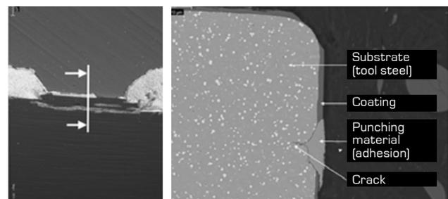
counteracting the formation of cracks, the associated material adhesion in coating gaps and thus the risk of chipping. FeinAI's proven high abrasion resistance had to be maintained while further optimising the coating system's crack resistance.
