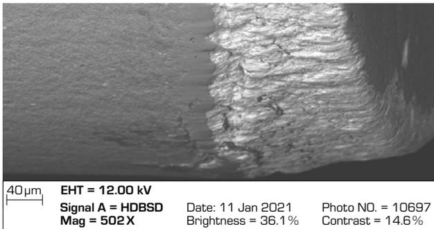
In most cases, active elements fail due to a combination of the main wear mechanisms: fatigue, adhesion and abrasion. Once a crack has started, crack propagation proceeds relatively quickly and leads to chipping of the cut edge. In brittle materials, chipping can occur over a large area. Such largescale damage usually requires immediate tool replacement or reworking.
