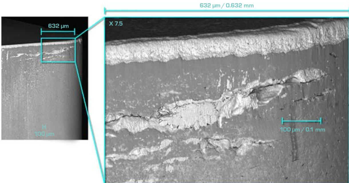
In addition to mechanical loads, increased temperatures also occur in the cutting edge area, mainly due to friction. There are indications that, depending on
