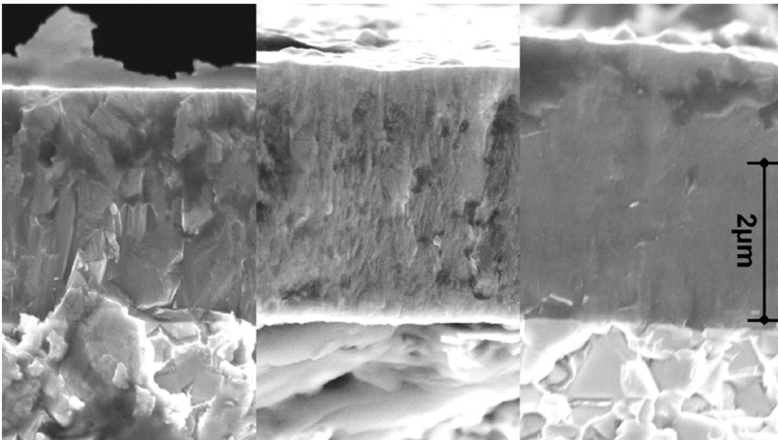
However, the most interesting effect of boron in the AlCr-based layer relevant to fineblanking is the reduction in the residual stress of the layer. The addition of boron increases coating hardness by around 15 %, while virtually halving the residual compressive stress of the coating, as the following graph shows. The higher coating hardness has a positive effect on abrasion resistance. Low residual coating stress improves crack resistance.
