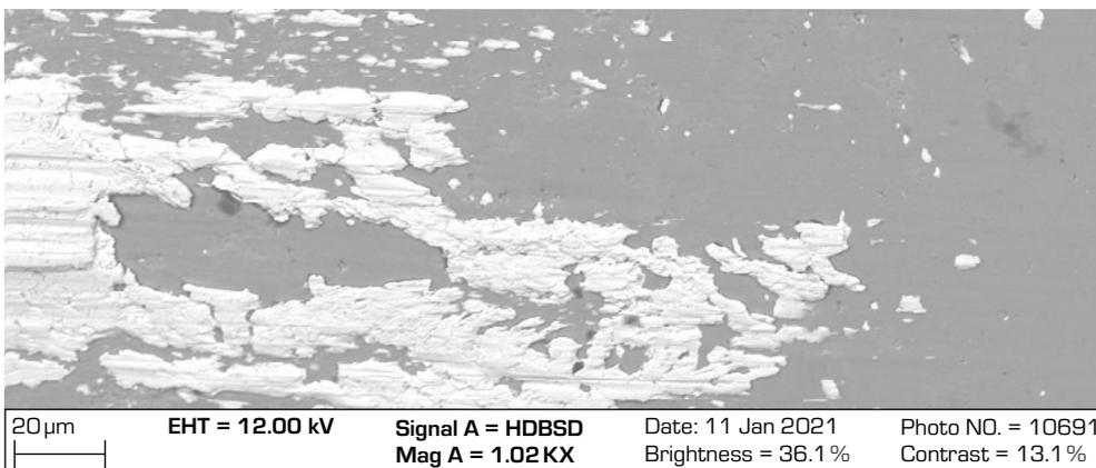
In addition to adhesive wear, hard particles in the punching material (e.g. carbides, nitrides and impurities) lead to abrasive wear. These hard particles cause microchipping under the relative movement of
