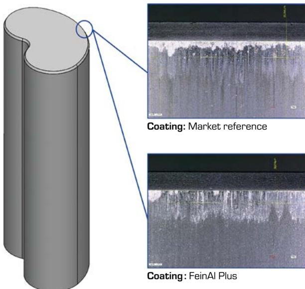
The wear images shown above were taken after 23,500 strokes. The two microscope images show wear patterns. Compared to the market reference, a reduction in cold welds is found with FeinAI Plus. This is associated with reduced fatigue cracks and consequently less visible wear on the inner punch.
