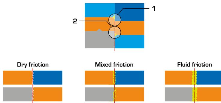
**Adhesive wear phenomena on the surface of a fineblanking die:**
