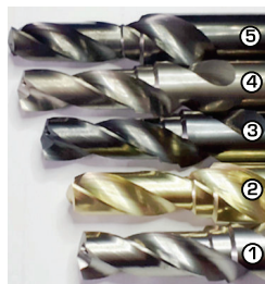
Tool: aluminum step drill; GIW/PCG Workpiece material: GD-AlSi9Cu3(Fe); 9.3 % Si Source: PLATIT AG and PannonPLATIT, Budapest, HU
