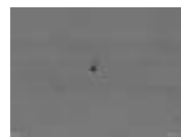
Material inhomogeneities (pores or carbides)
