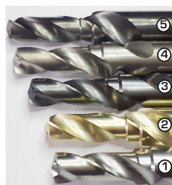
Tool: aluminum step drill; GIW/PCG Workpiece material: GD-AISI9Cu3(Fe); 9.3 % Si Source: PLATIT AG and PannonPLATIT, Budapest, HU
