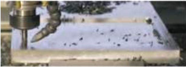
Fig. 5: BorAC® AlCrN/BN: Cutting Performance at Milling.
