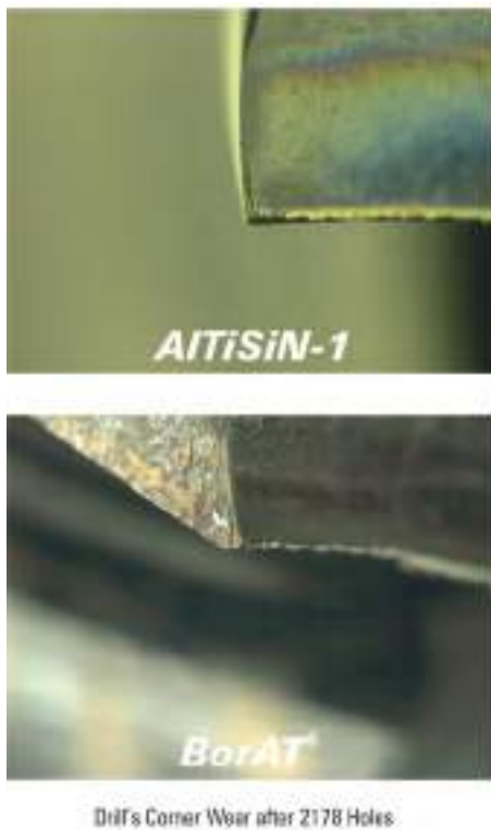
Fig. 7: BorAT® – AlTiN/BN: Wear Behavior at Drilling.
