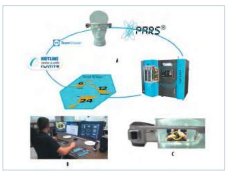
2 PARS-PLATIT Augmented Reality Service A: The on-line circle of PARS; B: The hotline service engineer is connected on-line with the coating machine and with the PARS glasses of the machine operator; C: The operator sees the markings and instructions of the hotline service engineer in his glasses (© Platit)
