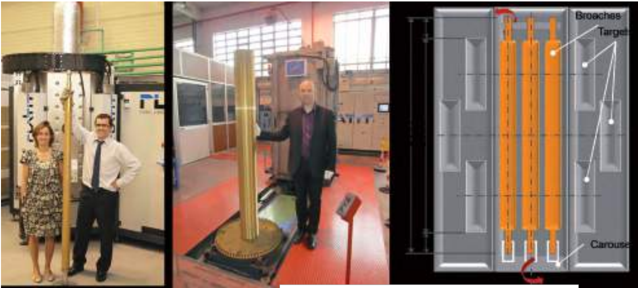
Fig. 6: Coating equipment for broaches A: PL1400 with hat at Metallestalki, Bilbao, Spain B: PL2500 at Genta, Torino, Italy C: PL2511 project with 6 cathodes
