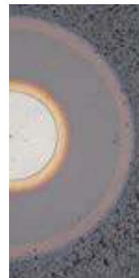
Calo 3 layers AlTi(Si)N is deposited on a TiN adhesion layer
