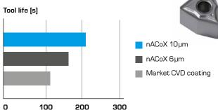
Tool: Turning insert WNMG 080412 Workpiece material: Ni-steel Coolant: MQL vc = 110mm/min; f = 0.4mm; ap = 0.2 mm Source: German automotive manufacturer
